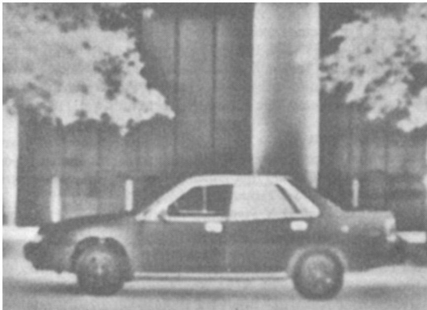
Fig. 4. Thermal image produced by the pyroelectric effect in ferroelectrics. The image was taken by a BST detector with NETD = 0.2 K and f/1.0 optics [14]. Recent detectors NETD = 0.02 K.
